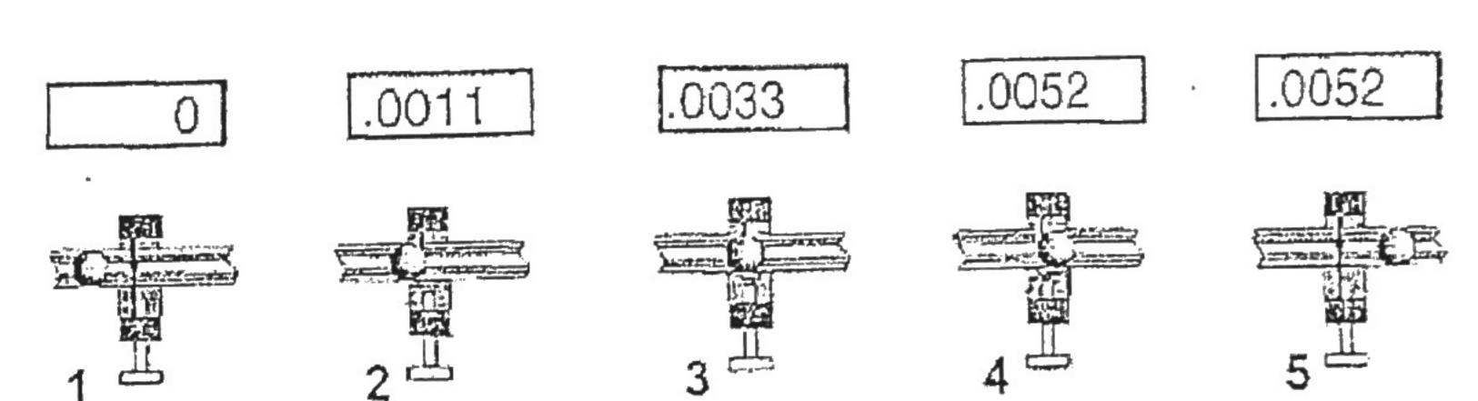
Speed is the distance traveled divided by time taken to travel that distance. During the time that the timer is counting, the cart wing is the distance traveled. The speed of the cart is the length of the cart wing (5 cm) divided by the time from photogate A.
